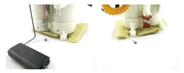
2 – pry the fuel sock off the pumps and then pull the base away from the assembly
