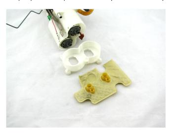
3 – disconnect the electrical connectors from the pumps and then pull the pumps out of the assembly
